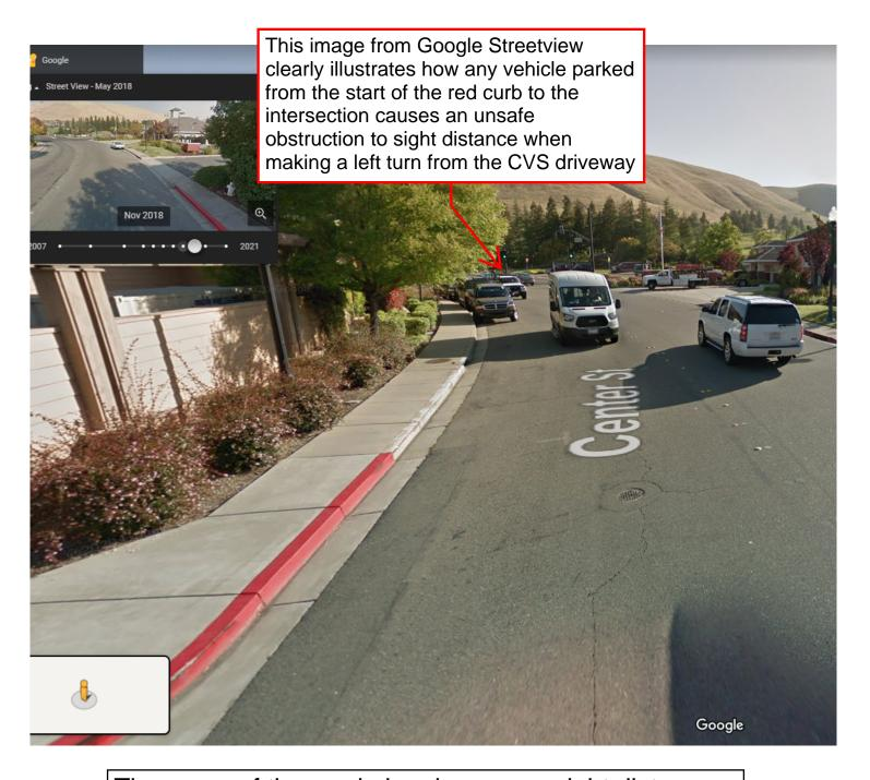
The curve of the road also decreases sight distance. The recommendation based on suggested sight distances for passenger cars entering two lane roadways from stop is to remove all parking - to paint curb red from existing limit to the intersection. Clayton Muni Code requires new red curb locations to be approved in City Council.
