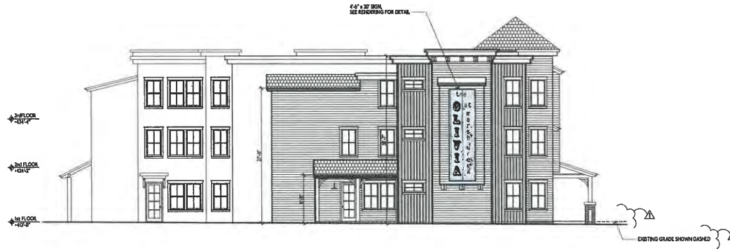
REAR (SOUTH) ELEVATION 1/8" = 1'-0"
